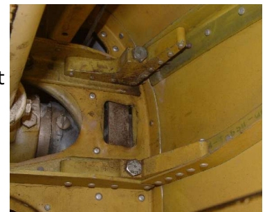
Torque tube mounting braces.
